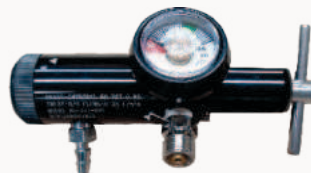
Ultra Pin Index with DISS Inlet pressure: 250 Bar Outlet pressure: 3 - 6 Bar Increments: 1,2,4,6,8,10,12,15,18,20,25 \text{Lpm}
